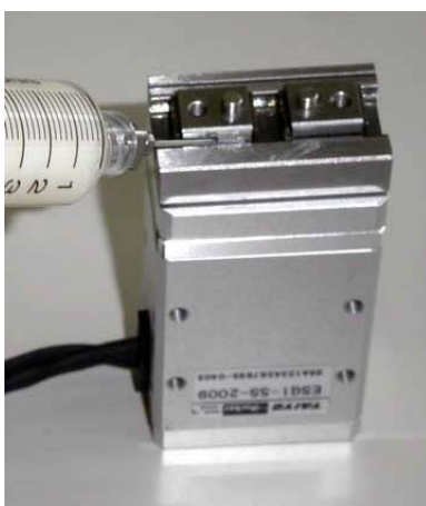
Fig.4-6:Applying grease to the guide part
