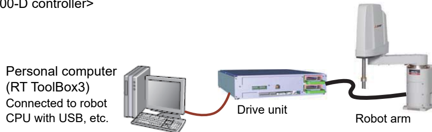
Fig.5-13: Connecting the devices (CR800-D controller)
