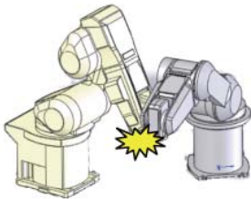
Fig.5-10: Interference check during robot operation (automatic operation, jog operation)
