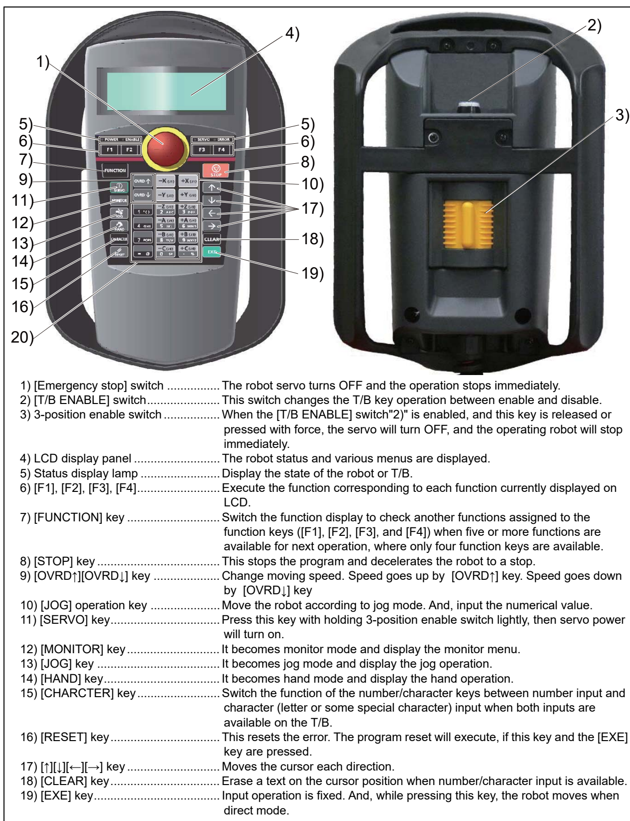
Fig.3-17: Teaching pendant key layout and main functions
