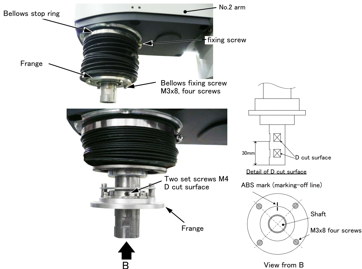
Fig.5-21 : Replace the bellows (oil mist specification)
