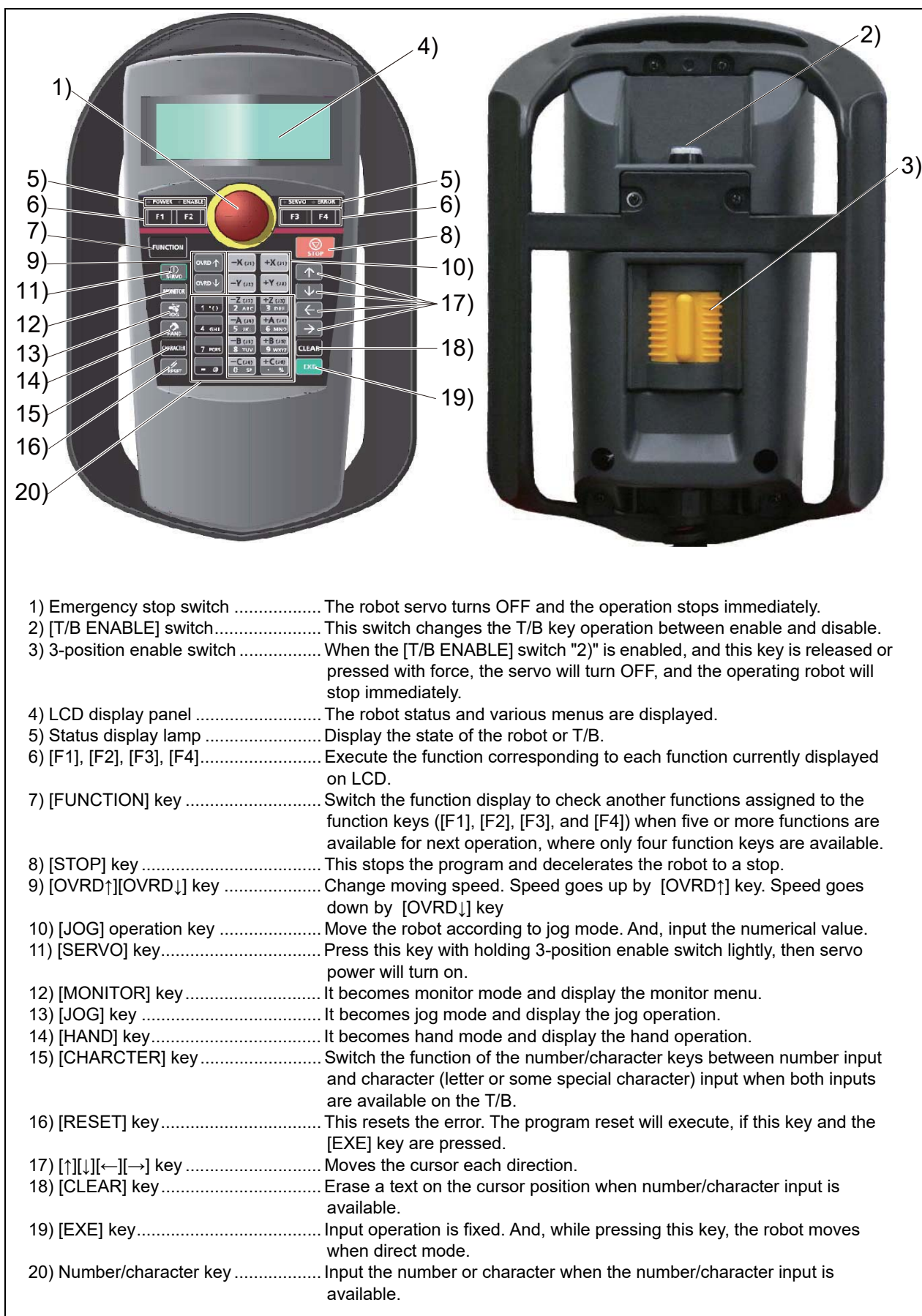
Fig.3-17: Teaching pendant key layout and main functions
