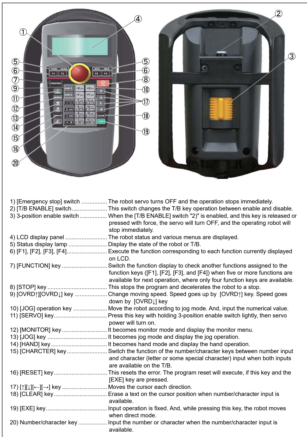
Fig.3-17: Teaching pendant key layout and main functions
