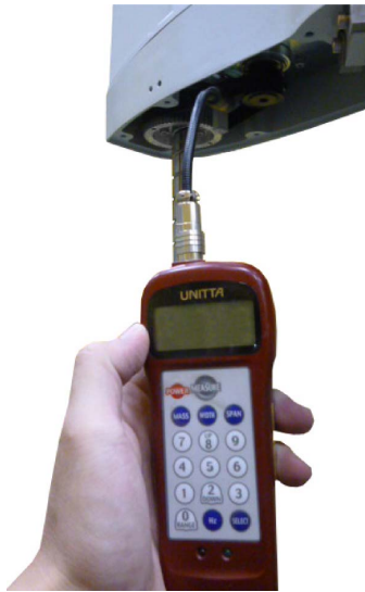
Fig.5-3:Tension adjustment method of timing belt
