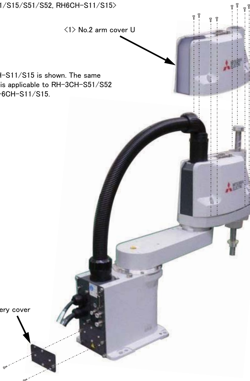
Fig.5-4 : Installing/removing the cover (RH-3CH-S11/S15/S51/S52, RH-6CH-S11/S15)
