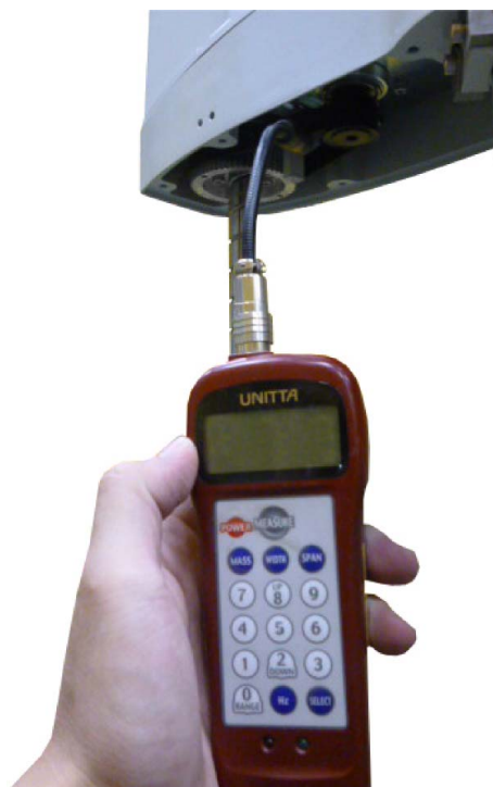
Fig.5-9 : Tension adjustment method of timing belt
