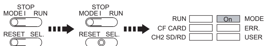
Figure 16.28 Switch operation for the hardware self-diagnostics mode (for the Q06CCPU-V)
